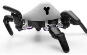
Six-legged robot (Hexa): Able to scale steps and balance on uneven ground
